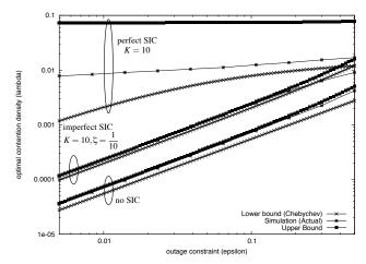
Fig. 5. Optimal contention density  $\lambda^{\epsilon}$  versus the outage constraint  $\epsilon$  for the no SIC, imperfect SIC, and perfect SIC scenarios.
