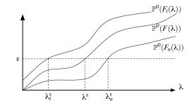
Fig. 2. Illustration of the technique to find lower and upper bounds on the contention density:  $\lambda_l^\epsilon \leq \lambda^\epsilon \leq \lambda_u^\epsilon$  through the use of necessary and sufficient events for outage.
