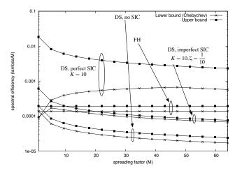
Fig. 9. Spectral efficiency  $\lambda^{\epsilon}/M$  versus the spreading factor M for four scenarios: DS-CDMA with no SIC, DS-CDMA with imperfect SIC, DS-CDMA with perfect SIC, and FH-CDMA.
