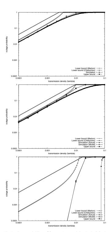
Fig. 4. Outage probability  $p_o(\lambda)$  versus the transmission density  $\lambda$  for the cases of no SIC (top), imperfect SIC with K = 10 and  $\zeta = \frac{1}{10}$  (middle), and perfect SIC with K = 10 (bottom). All three plots show both the Markov and Chebychev "lower" bounds and the "upper" bound, as well as simulation results with confidence intervals.
